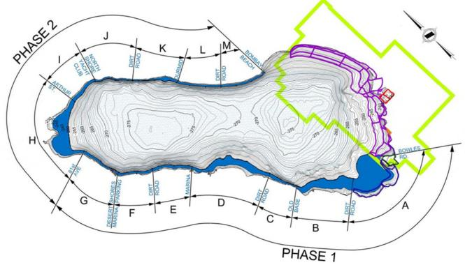
Figure 16: Access Levee Locations and Construction Phases
